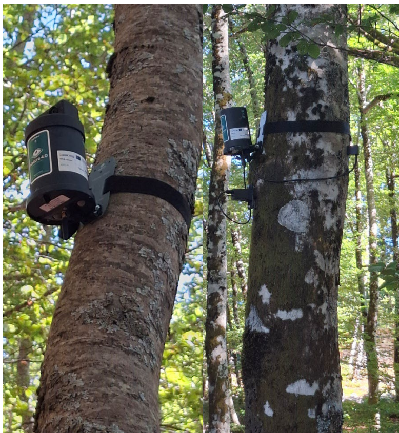
Figure 2. TreeTalker Fire and TreeTalker Cyber sensors installed on trees at the Jezerski Vrh and Ivanova Korita monitoring sites.
